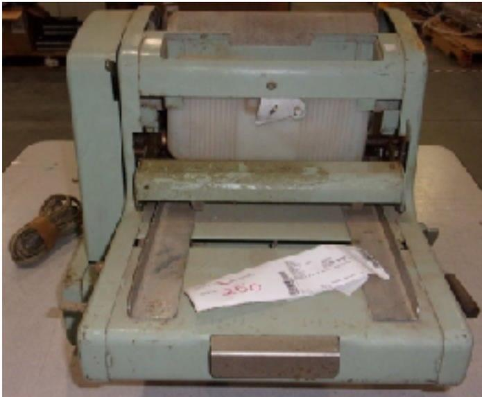
reproducing handouts required one to type a Ditto Master, a two sided affair with the second sheet being a carbon copy on special paper. The carbon was then detached from the original and affixed to the cylinder of the Ditto Machine (Spirit Fluid Duplicating Machine), which when rotated by hand, produced the number of copies desired. Fluids were automatically added to this production,
